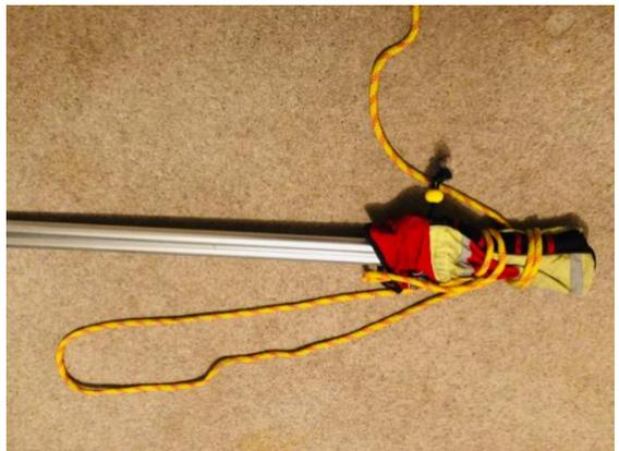
When tightening the stays for the A Frame, ensure the A frame is slightly leaning backwards, as the force of the wind in the sail will pull the poles forwards a little bit. Leaning back to start off with will counter this. Also, the Front stay wants to be to the centre thwart so that the sail can be free to fly in front of it.
